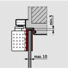
**Glass door saddle plate for TS 92** For fixing the closer to toughened glass doors – No glass drilling or recessing required.
