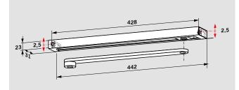
The **G-N** slide channel assembly comprises the main arm, slide channel, slide block, fixings, screws and end caps. The G-N slide channel is non-handed and can be combined with both door closers. Thanks to oblong holes in the fixing pads, it is possible to compensate for deviations in the drill hole pattern and to keep the door closer body and slide channel perfectly parallel.
