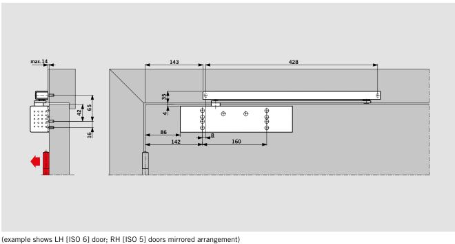
Provided the structural conditions allow, an opening angle of 180° is possible with this method of fixing. In most cases, however, a wall recess will have to be provided for the door closer.
