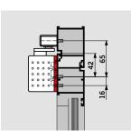
Mounting backplate for TS 91 For fixing to doors which provide no means of direct mounting. Fixing hole pattern as per Supplement 1 to EN 1154.
