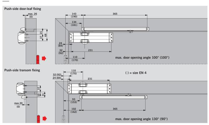
Depending on the structural conditions, the door opening angle is likely to be limited. It is recommended to install the cushioned limit stay or position a door stop at this point.
