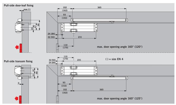
Depending on the structural conditions, the door opening angle is likely to be limited. It is recommended to install the cushioned limit stay or position a door stop at this point. A door stop must be installed in the case of fire and smoke check doors.
